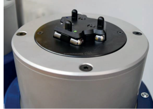
Measuring head with measuring ball inserts and distance bolt
