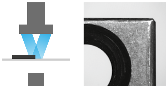
▲ Principle of incident light measurement: The resulting image additionally shows detailed surface features – such as the chamfer of the bore shown in the picture.
